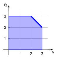
Each transmitter (nodes 1 and 2) may transmit at rates  $r_i = 2$  without having any influence on the transmit rate of the other source, i.e., without utilizing the shared link (3, 4). Without loss of generality let node 1 fully utilize that shared link, which allows to transmit at rate  $r_1 = 3$ . The second node may still transmit at rate  $r_2 = 2$ . For  $2 < r_1 \le 3$  the residual capacity on the shared link may be utilized by node 2 such that  $r_1 + r_2 = 5$ .
